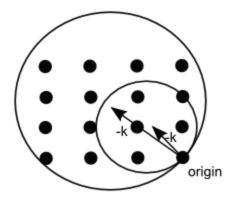
• Tilt the sample, which drags the reciprocal lattice around the origin without affecting the Ewald sphere
